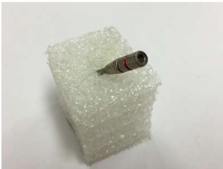
Figure 3.2 : Photograph of 5 \mu\text{Ci} ^{226}\text{Ra} standard radiation source.
