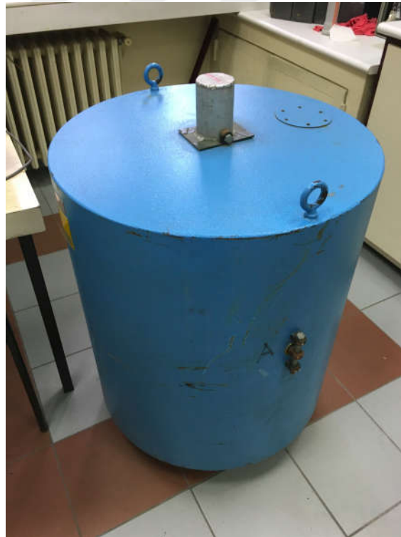
Figure 1.1 : Photograph of 3 Ci Am-Be neutron source from J.L. Shepherd and Associates.
