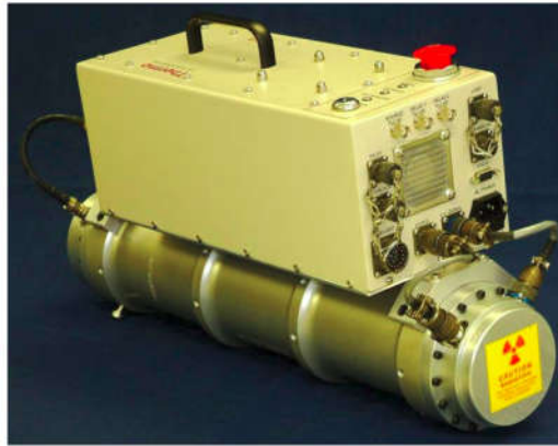
Figure 1.2 : The Photograph of Thermofisher MP320 Neutron Generator [3].
