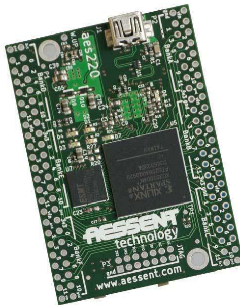
Figure 2.11 : AES220B Spartan 3AN FPGA board from Aessent Technology [18].
