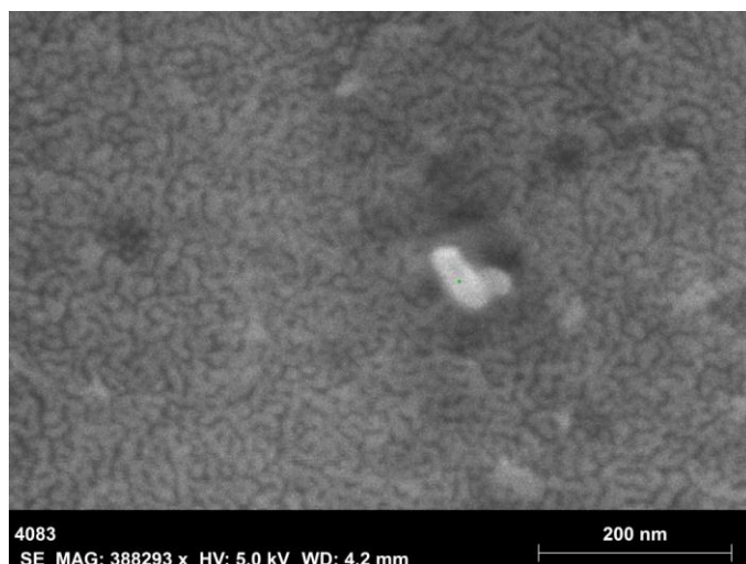
Figure 5.18: Image of EDX applied surface of PMMA with 5 (wt.%) borax.
