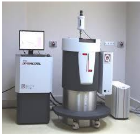
Figure 3.15: Quantum Design Model: PPMS DynaCool-9 [173].
