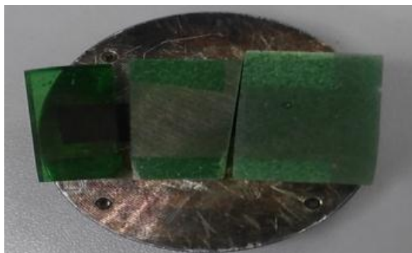
Figure 4.16: Coating of surfaces with gold.
