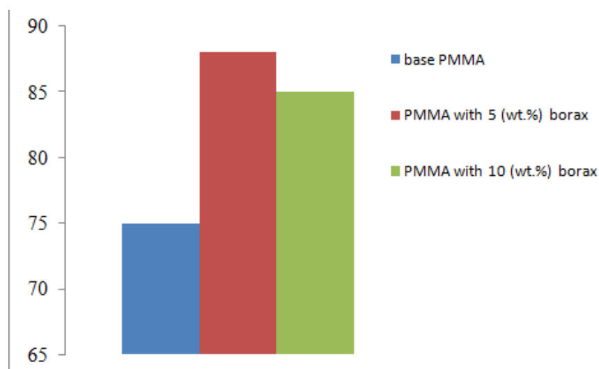
Figure 5.24: Shore D Hardness of base and composite samples in this study.
