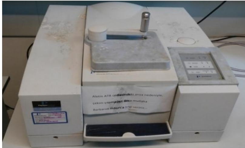
Figure 4.12: FTIR Spectrometer device branded PerkinElmer used in this study.
