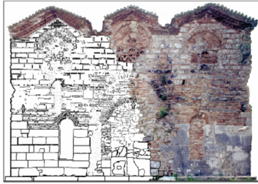
Figure 8. Photoplan of the monastery west facade with a partial vector drawing (reduction from 1:50 scale plot).
