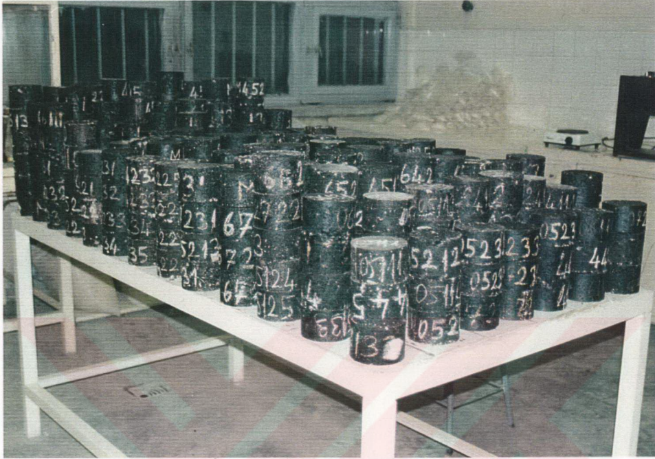
Figure 5.92 Specimens prepared for marshall and resilient modulus tests
