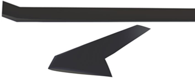
Figure 6.22 : UH60 Black Hawk blade geometry.
