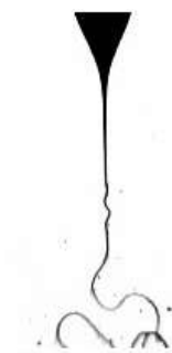
Figure 1.1. Electrospinning jet-Whipping Instability (Schultz, 2008).
