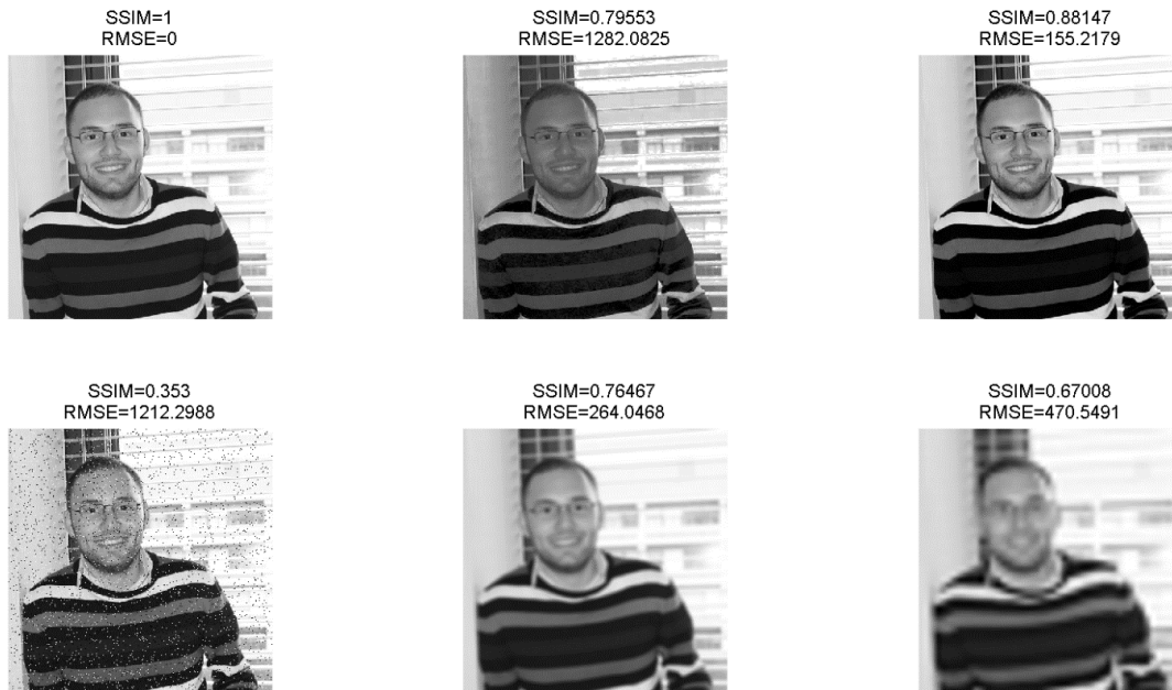
Figure 5.13 : SSIM & RMSE results a) Original b) Histogram equalized c) Contrast adjusted d) Salt & Pepper effect e) Blurred f) JPEG converted.
