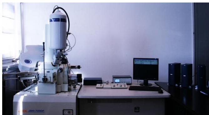
Figure 2.2: Field emission scanning electron microscope, JEOL JSM 7000F.
