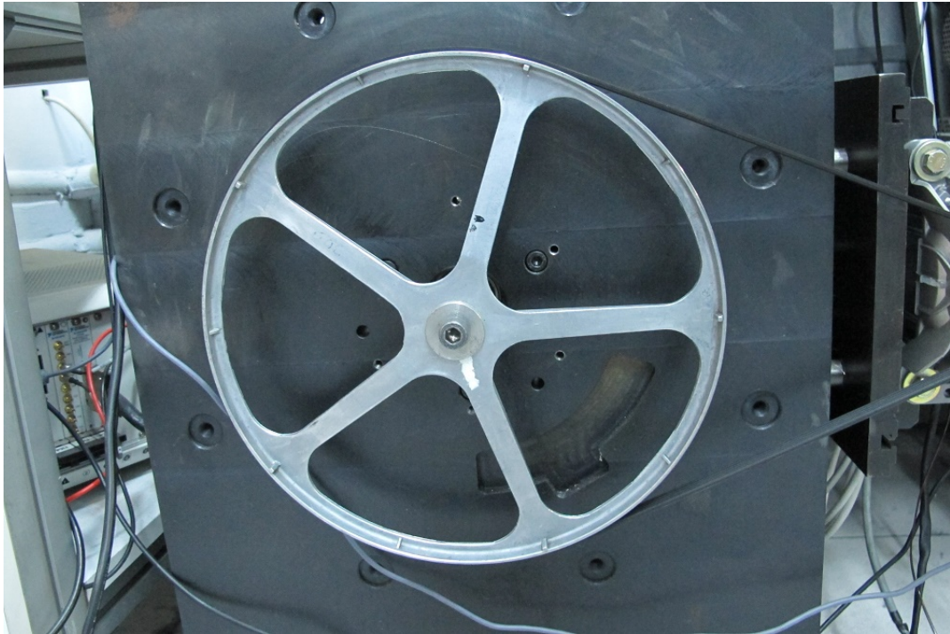
Figure 4.6 : The pulley connected to the hysteresis brake shaft.
