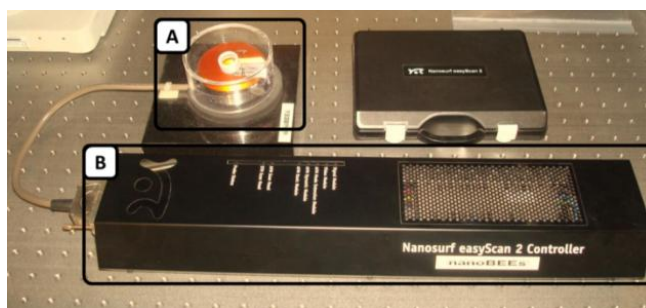
Figure 3.1: Nanosurf Easy Scan 2™ STM System for student educational purpose consists of an STM head (A) and an STM control electronics (B).
