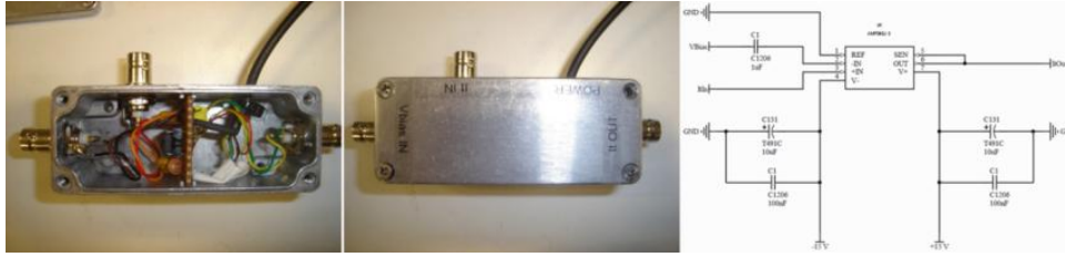
Figure 3.19: Bias voltage subtractor box and circuit schematic
