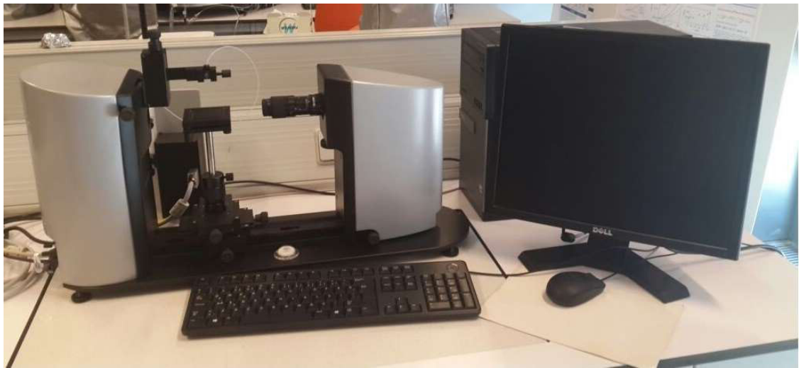
Figure 3.2 : Video recorder with high frame rate for contact angle measurement.
