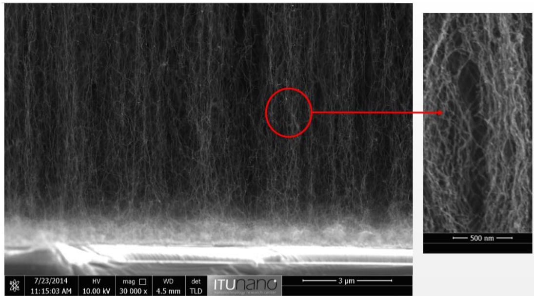
Figure 3.9 : An example SEM images of A-CNTs synthesized by CVD method.
