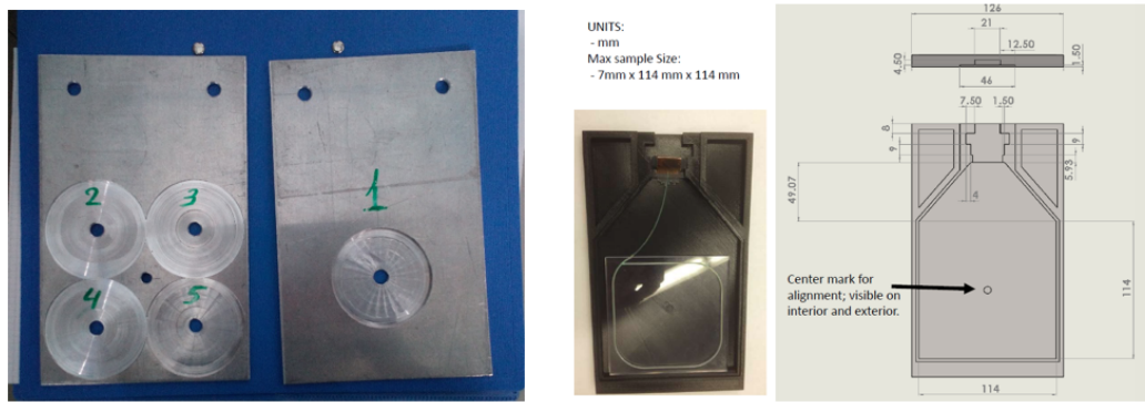
Figure 5.5 : (a) Source position for measurements. Sr-90 beta source are placed at 5 different positions one by one as indicated in the figure. (b) Tiles are put into black 3D-printed Wetzel boxes during measurements.
