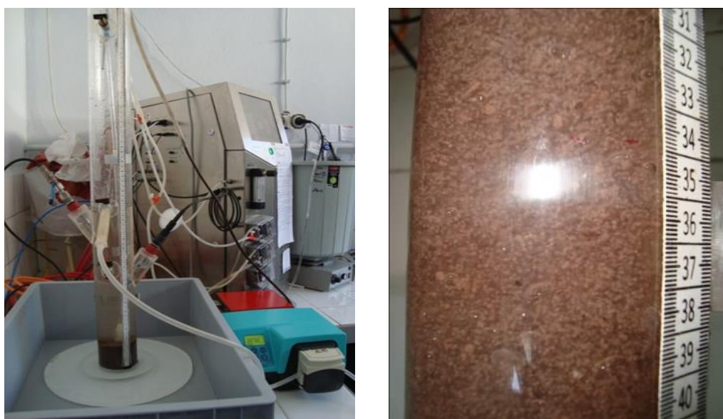
Figure 4.1: (a) Column SBR set-up (b) Granules in the column SBR.
