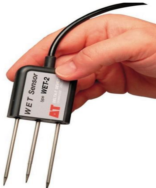
Figure 2.10: Soil salinity sensor (Url-5).
