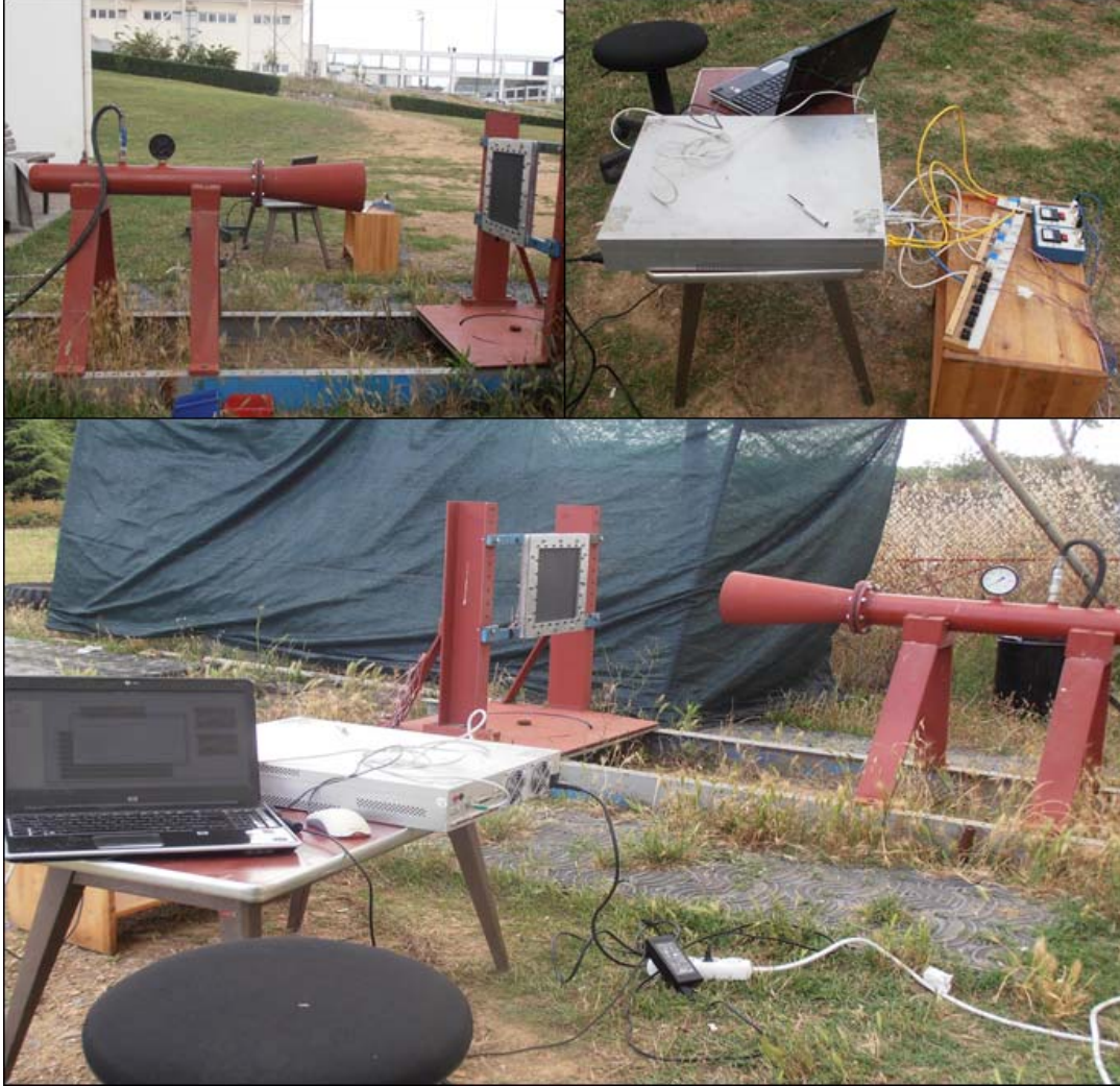
Figure 4.25 : General views of the tapered sandwich plate just before subjecting to air blast load.
