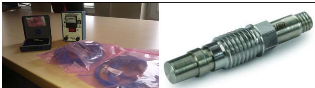
Figure 4.10 : The pressure sensor with signal conditioner and cables.
