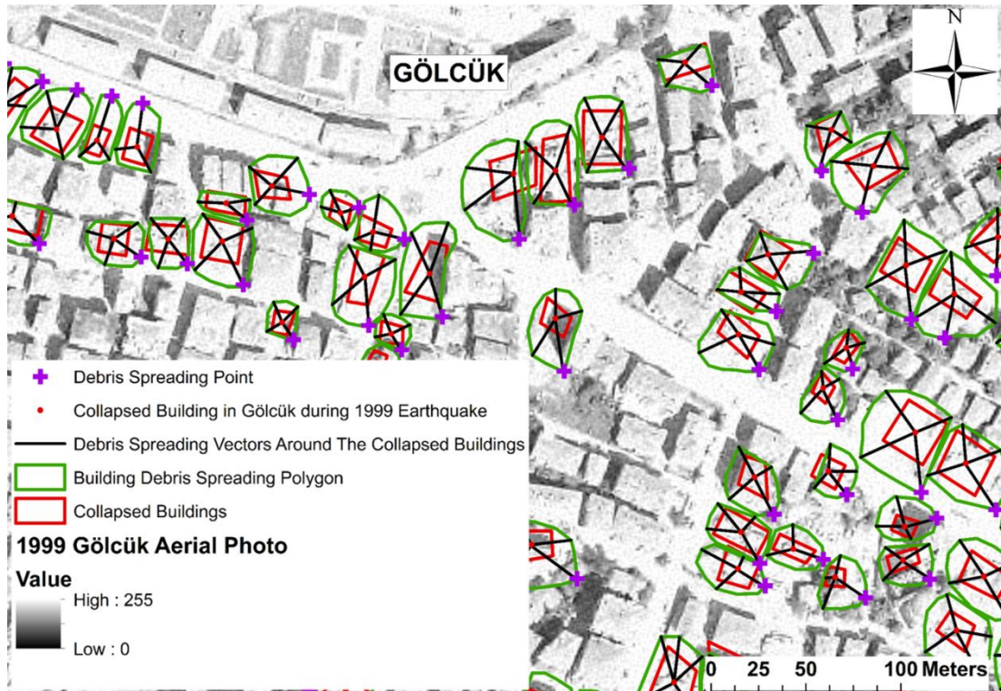
Figure 7.18 : Debris spreading vectors around the collapsed buildings in Gölcük.
