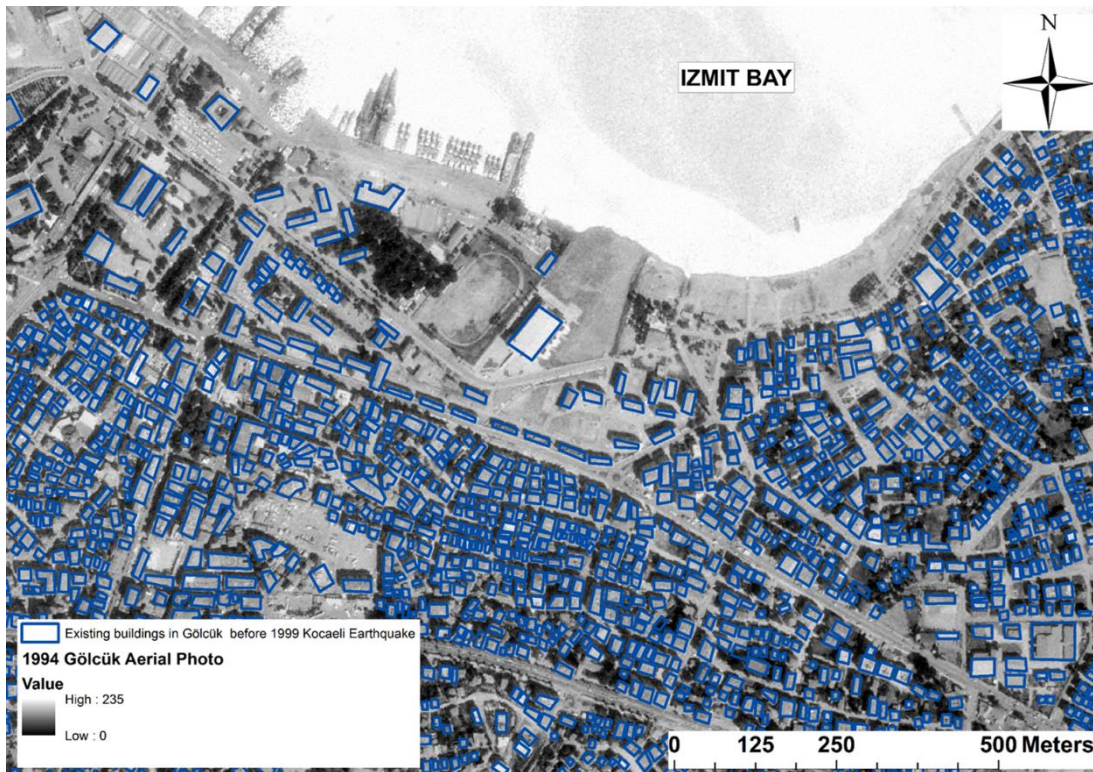
Figure 7.3 : The buildings that were built before 1994 in Gölcük.
