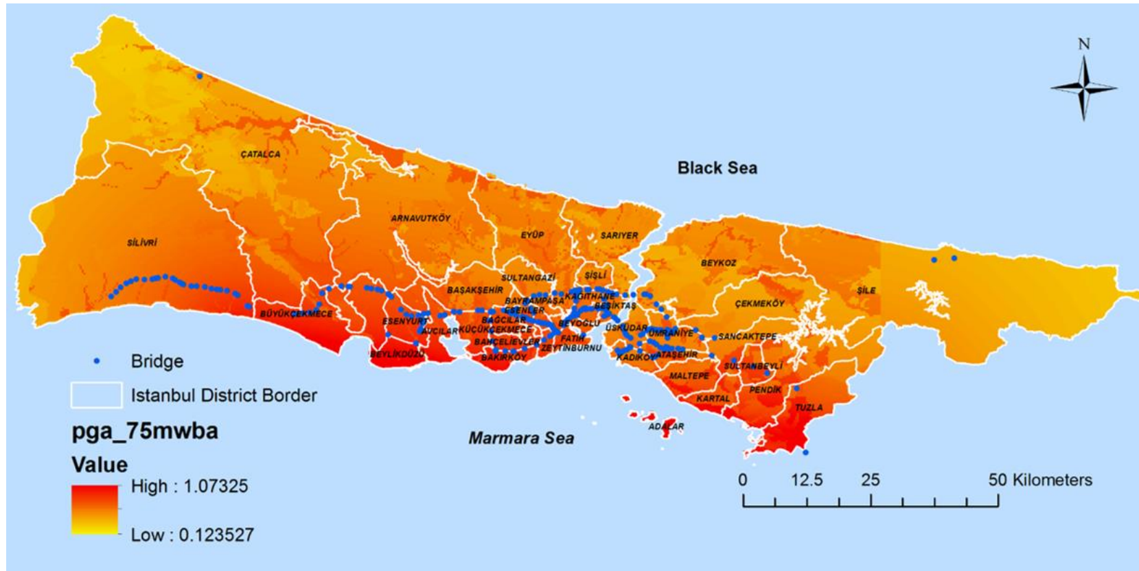
Figure 8.2 : Distribution of bridge locations on Istanbul Earthquake Hazard Map according to Boore & Atkinson (2008) PGA.
