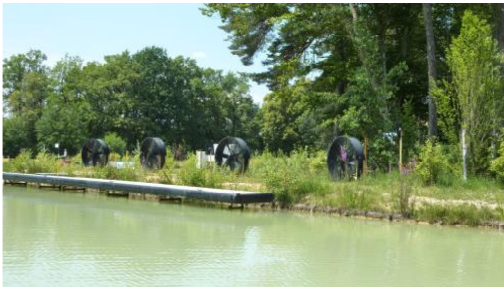
Figure 3.10 : Wind generators in Port Revel, photograph from (Ofdağ, 2013).
