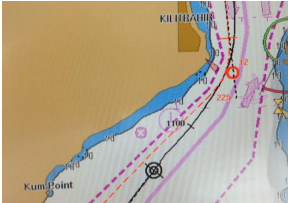
Figure 2.38 : ECDIS view of southbound Kilitbahir turn.
