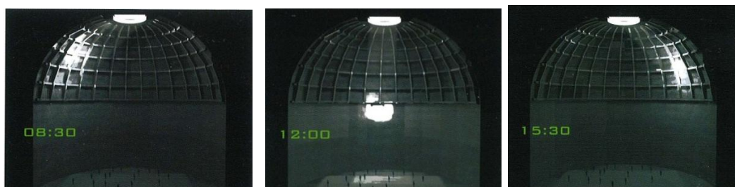
Figure 3.38 : Dialux visualisation of Pantheon showing the relationship with natural light under clear sky conditions ( Uyan, F. , p.57).
