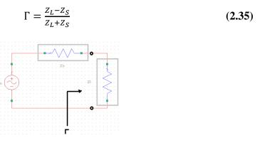
Figure 2.28 : Simple circuit configuration showing measurement location of reflection coefficient.
