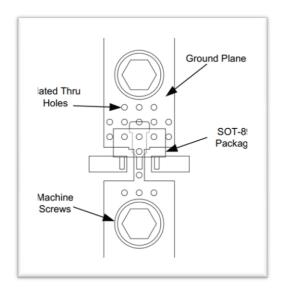
Figure A.2 : Recommended mounting configuration.
