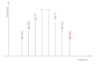
Figure 2.20 : Two tone intermodulation products.
