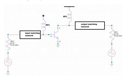
Figure 2.53 : The single-stage PA with matching circuits.
