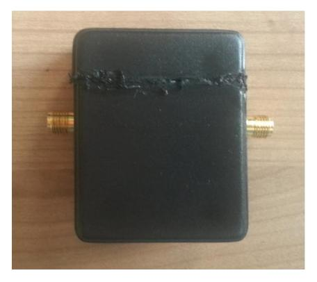
Figure 3.15 : Final version of the power amplifier.
