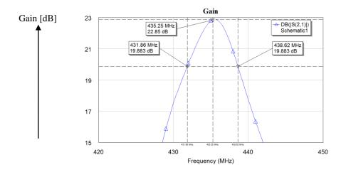
Figure 2.4 : Gain graph of a power amplifier.
