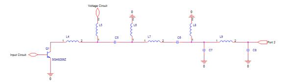
Figure 2.55 : The output matching circuit.
