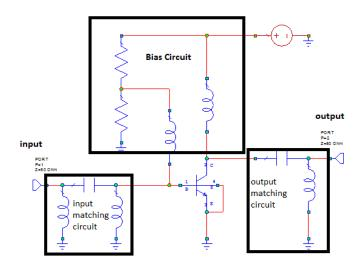
Figure 2.1: Schematic view of a basic RF amplifier.
