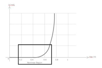
Figure 2.32 : Transistor's nonlinear region.
