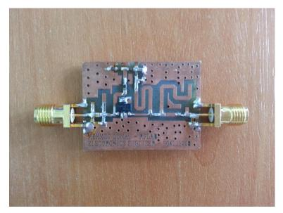
Figure 3.11 : PCB with Components.
