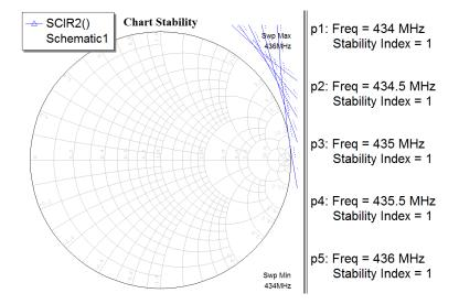
Figure 2.12 : The output stability circles.
