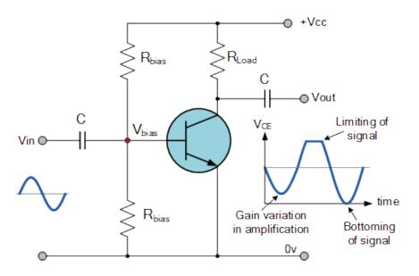
Figure 2.15 : Amplifier circuit distortion [Url-6].
