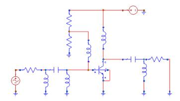
**Figure 2.2 :** Schematic view of a basic RF power amplifier with input and output impedances.
