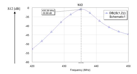
Figure 2.27 : The power amplifier's S<sub>12</sub> graph.
