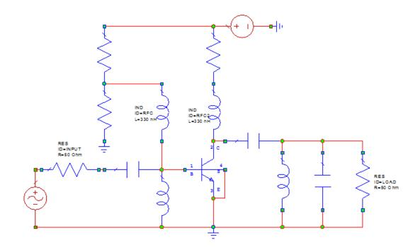
Figure 2.35 : The basic schematic version of Class A.
