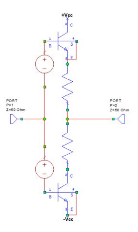
Figure 2.42 : The Class AB schematic.
