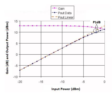
Figure 2.5 : 1 dB compression point characteristics [Url-14].
