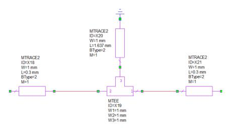
Figure 3.1 : The transmission lines.
