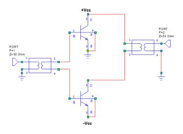
Figure 2.38 : The Class B push-pull power amplifier.
