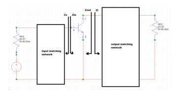
Figure 2.52 : An amplifier schematic showing Zin, Zout, ZL and Zs.
