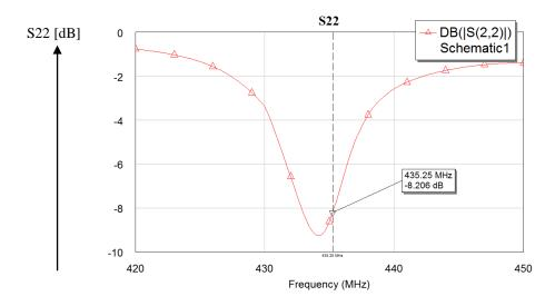
Figure 2.25 : The power amplifier's S<sub>22</sub> graph.
