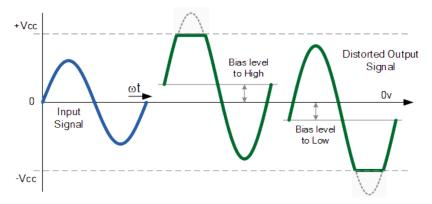
Figure 2.16 : Amplitude distortion due to incorrect biasing [Url-6].
