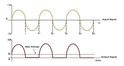
Figure 2.40 : The conduction angle of Class AB power amplifier.
