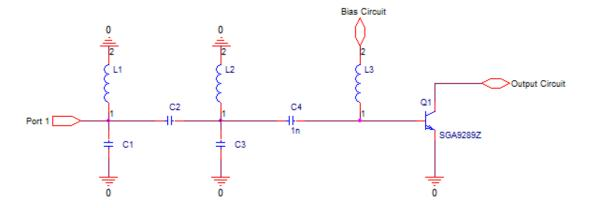
Figure 2.54 : The input matching circuit.
