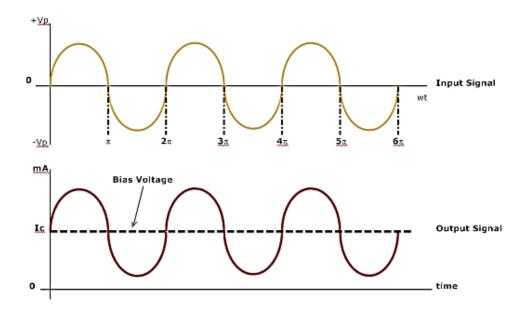
Figure 2.34 : Class A input and output wave form.
