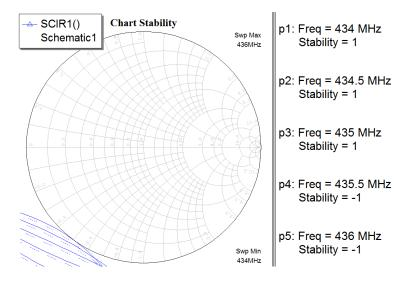
Figure 2.11 : The input stability circles.
