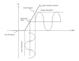
Figure 2.33 : Class A input and output wave form.
