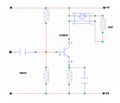
Figure 2.36 : The transformer coupled Class A power amplifier.
