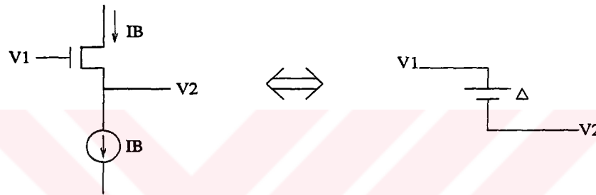
Figure 3.3: The idea of using a level shifter to reduce the equivalent threshold voltage
