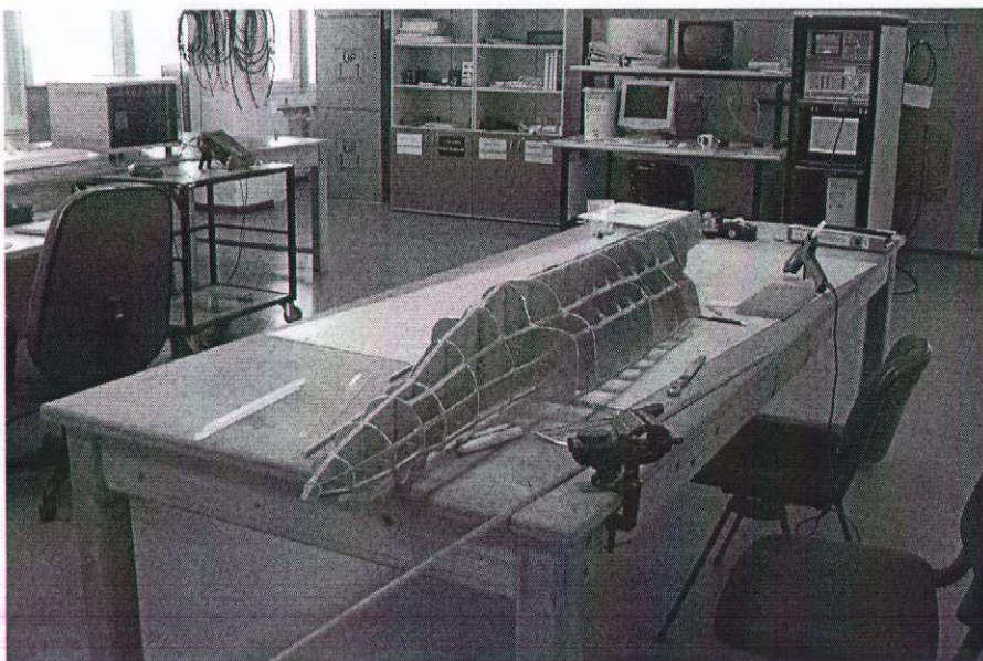
Figure 5.3: Reinforcing the model by long narrow strips of wood
