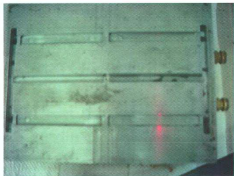
Figure 3.4 flexural specimen mold according to ISO178 standard
