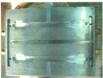
Figure 3.5 tensile specimen mold suitable to produce specimens with weld-line according to ISO R527 standard
