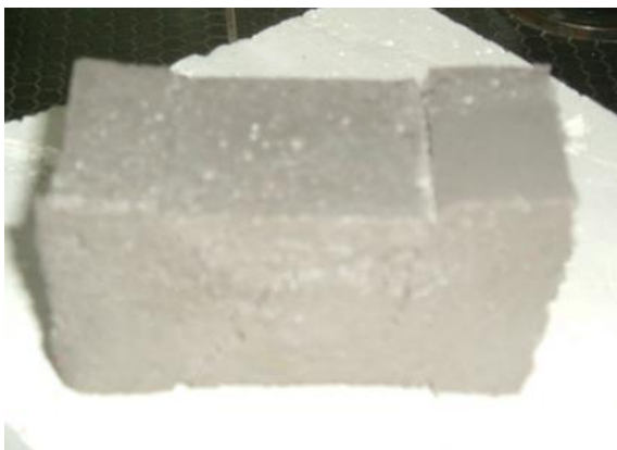
Figure 6.1: Sample including hardener 4 and 30% benzyl alcohol ,after compression.
