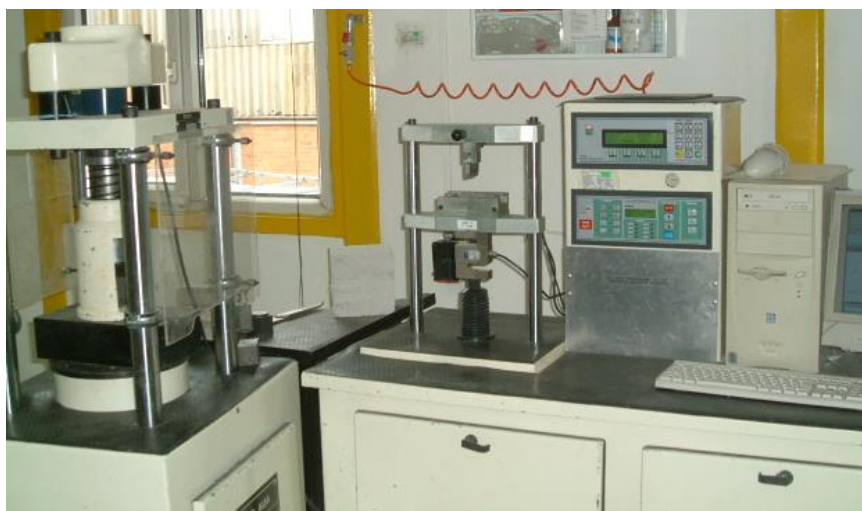
Figure 4.5: Alşa Laboratory Equipment on which the bending and compression tests were made
