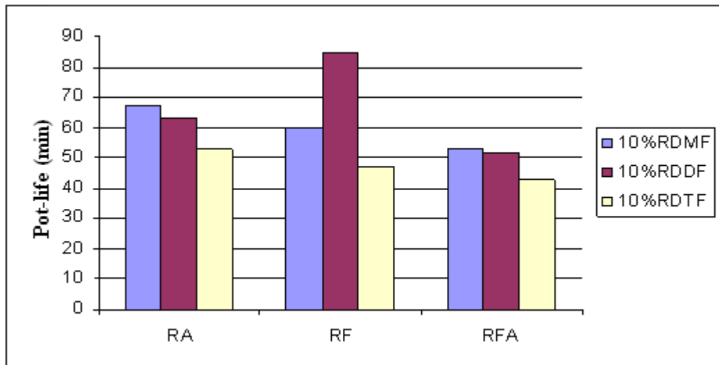
Figure 5.10: Pot-life comparison for hardener 6 mixtures with different resin types.
