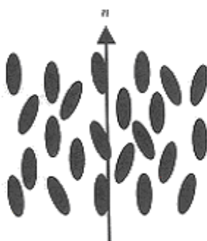
Figure 2.9 The structure of the nematic phase.
