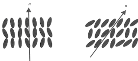
Figure 2.11 The smectic A and C phases
