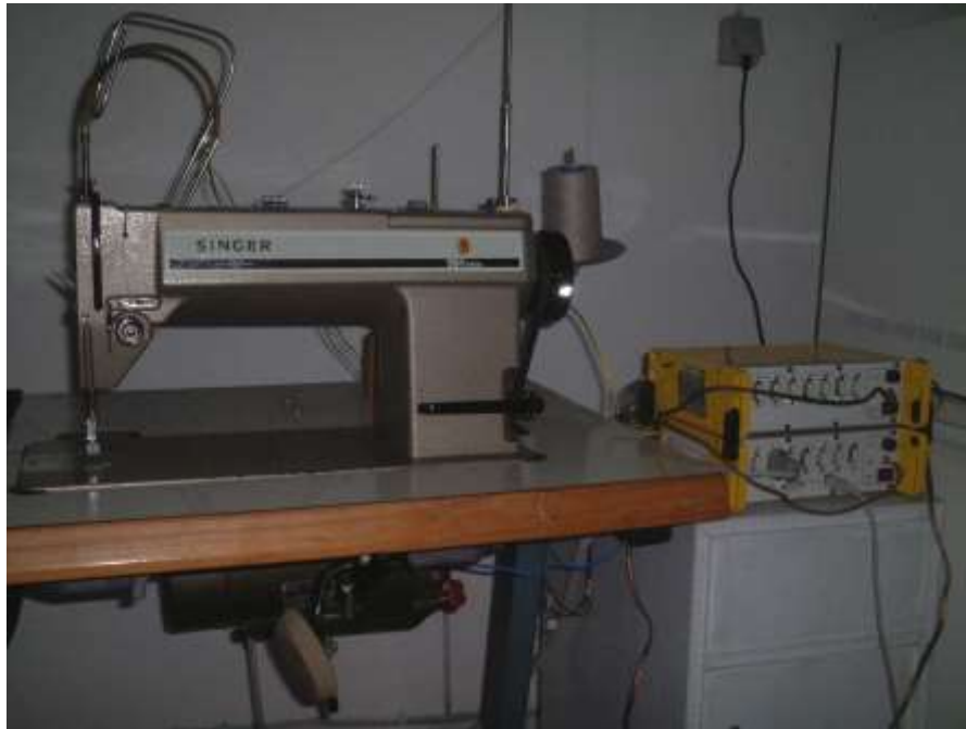
Figure 7.3 Sewing machine and ESAM Traveler amplifier unit
