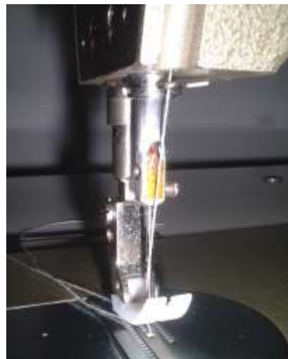
Figure 7.1 A close look to HBM strain gauge on the needle bar.
