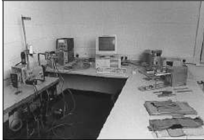
Figure 5.26 The intelligent lockstitch sewing machine integrated with fabric measurement systems
