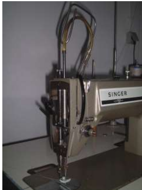
Figure 7.5 Side view of sewing head and needle bar arrangement
