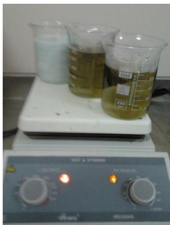
**Figure 3.2 :** Mixing and heating of precursors with different chelating agents on magnetic stirrer.
