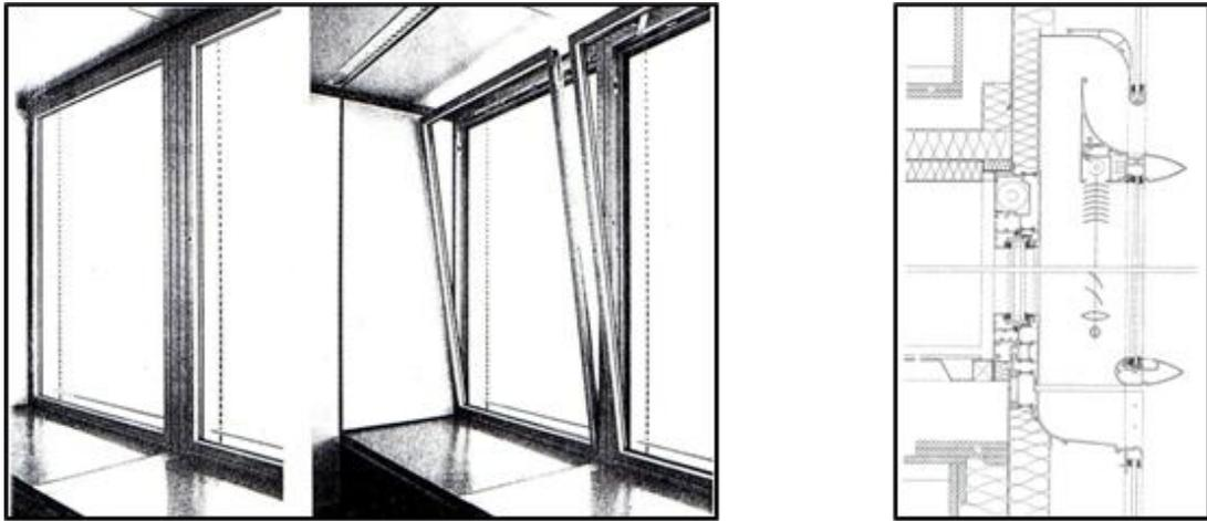
**Figure 3.17 :** Operable windows allowing natural ventilation with double skin, adapted from Davey (1997a).
