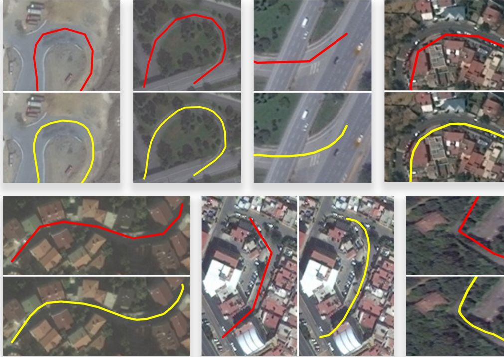
Figure 3.6 : A visual comparison of proposed curve fitting approach (yellow line) with existing linear approach (red line).
