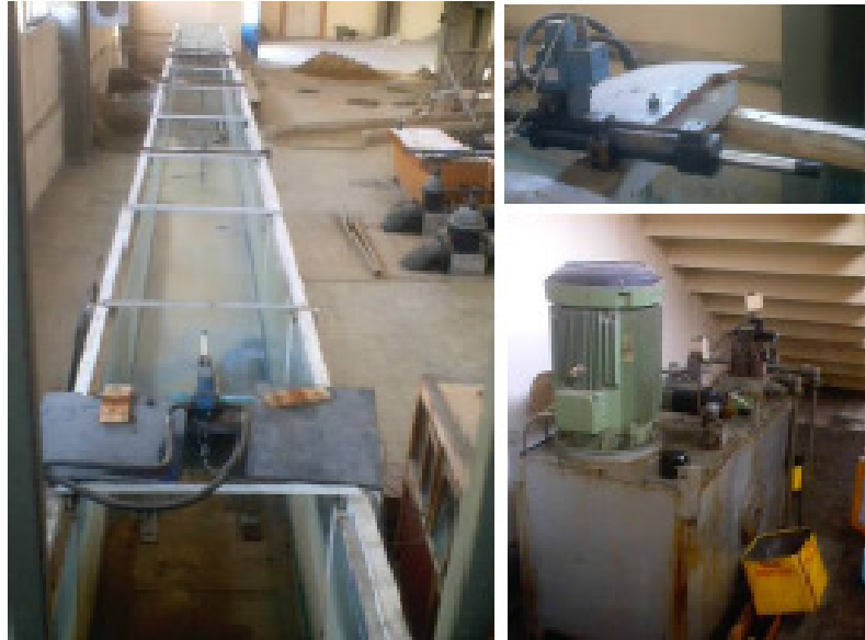
Figure 4.1 : Top view of the wave flume, hydraulic ram of the wave paddle and the hydroelectric power unit used during the tests.
