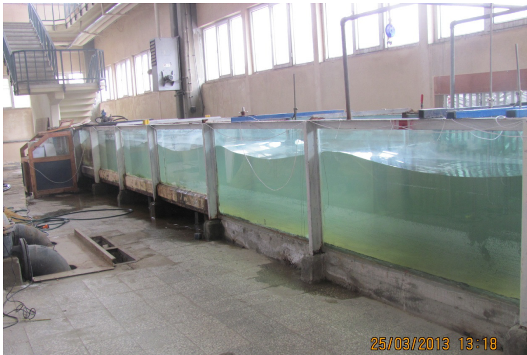
Figure 4.7 : A view of the wave flume during regular wave tests.
