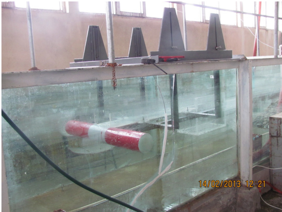
Figure 4.4 : Model shown in the channel fixed at the mounting frames.
