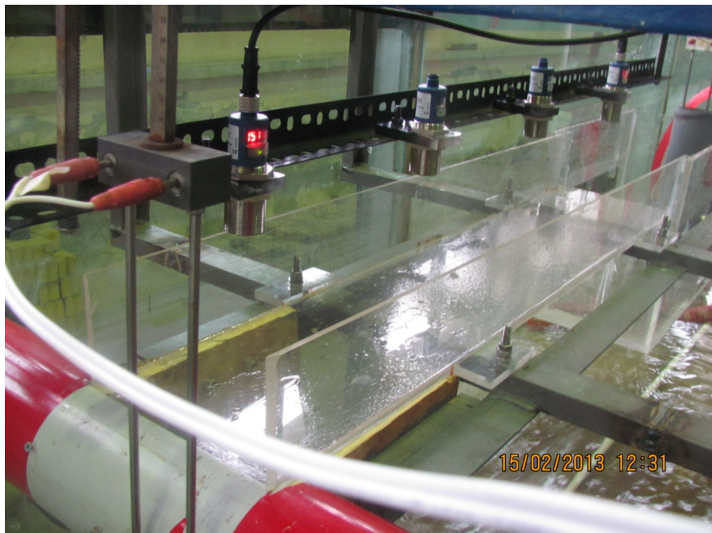
Figure 4.5 : A close-up view of the ultrasonic sensor installation.
